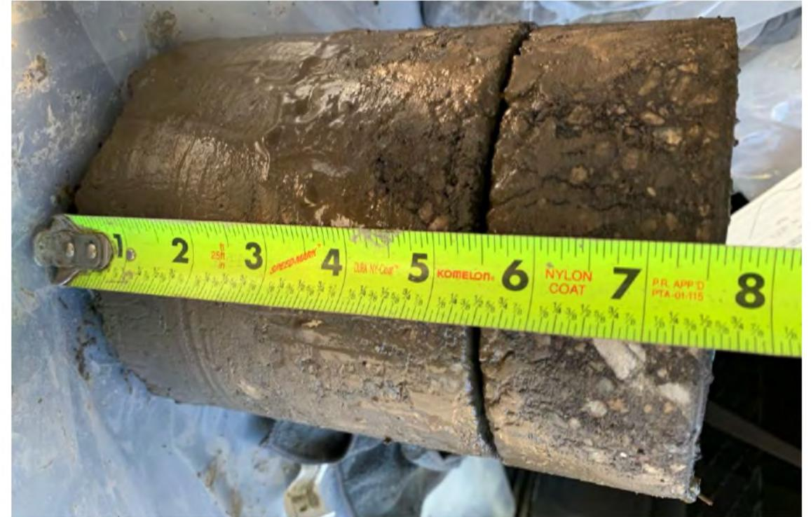
Photo 4: Core sample C-5 measuring 7.5 inches thick AC with an existing separated surface lift of 2.0 inches.
