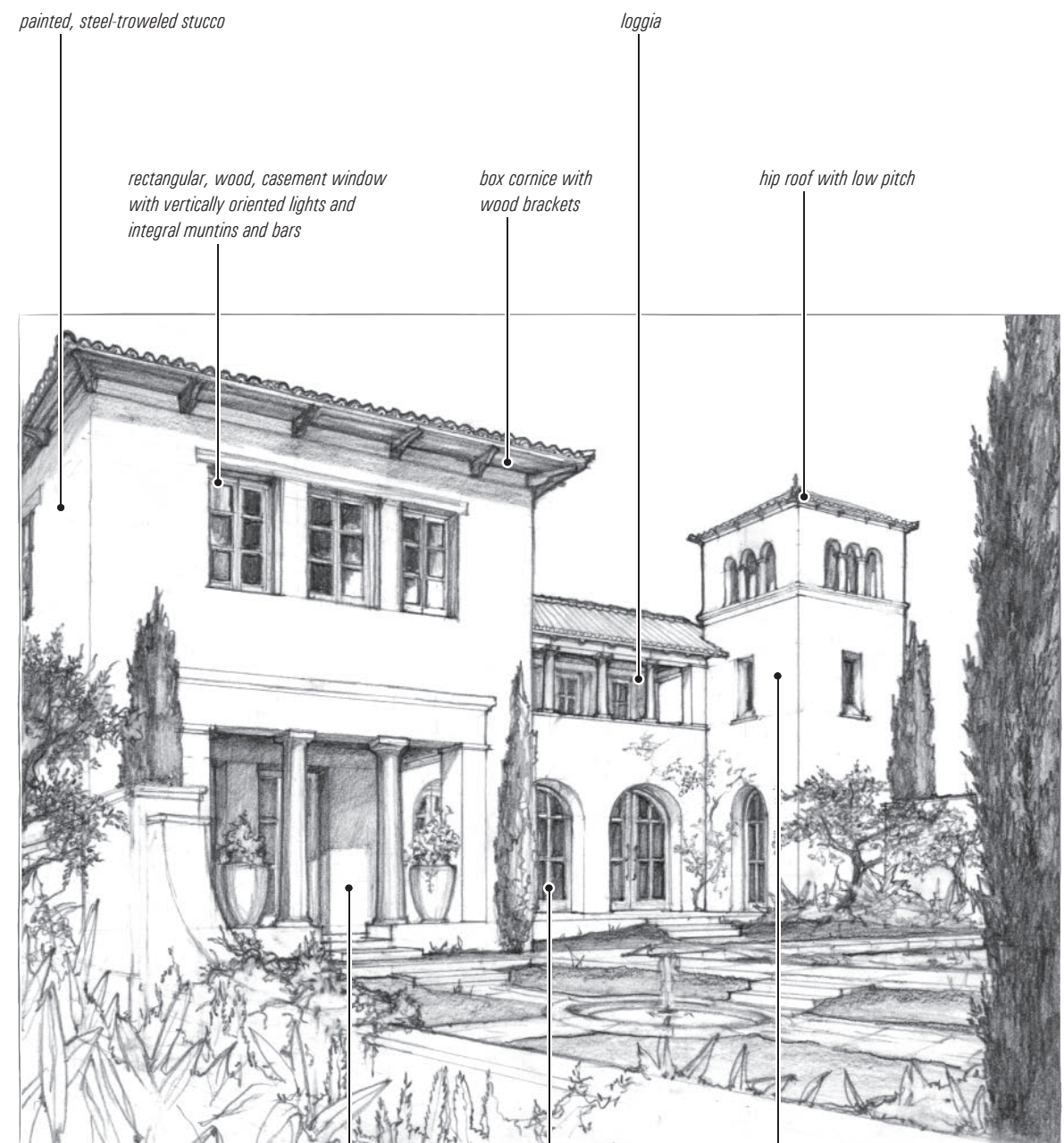
Italian Revival rear elevation
